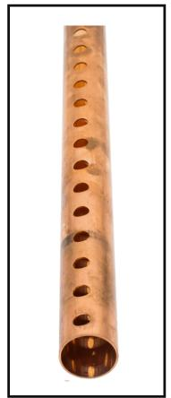
The operator loads the tube onto the mandrel and clamps the end of the tube in the indexing carriage. This carriage moves linearly and/or rotates the tube to positions defined by the linear template (spacer bar) and the rotation template (index plate). The punch is activated by a hand-operated valve. Slugs are automatically ejected by air pressure.
